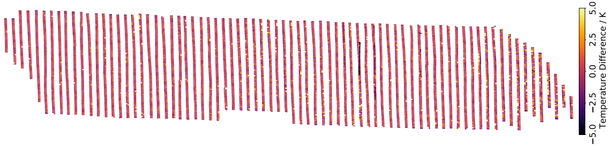
Figure 4.3: Map of a PV plant revealing anomalous PV modules by plotting trend-corrected maximum module temperatures. 1
